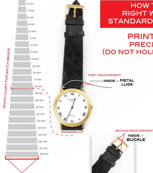
CAREFULLY MEASURE THE DISTANCE BETWEEN THE INSIDE OF LUGS & BUCKLE
